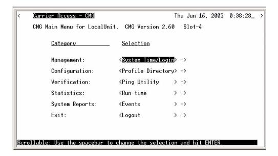
This screen provides the basic system and security options for the Router card.
